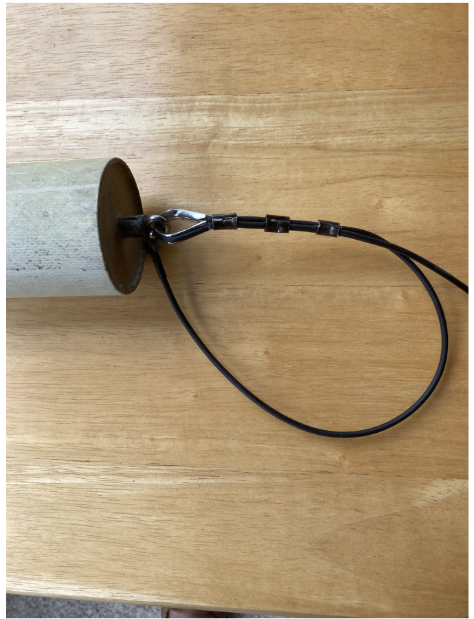
Figure 4 — Closeup of how the wire is connected to the balancing network. The balun was connected in the same way.
