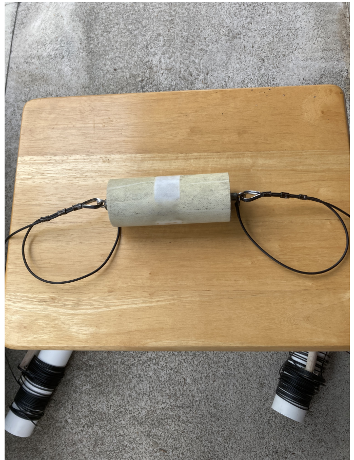
Figure 3 — Top wire attached to the balancing network with thimbles and ferrules. Each side of the antenna is rolled up onto 3-inch diameter plastic pipes for transport to the site.
