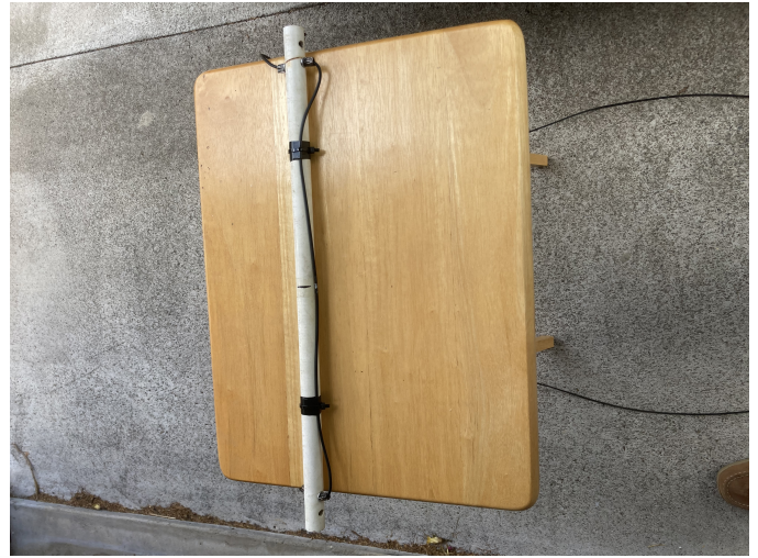
Figure 2 — It is important to align the center of the wire with the center of the end spreader before securing it with electrical tape, washers, and ferrules.
